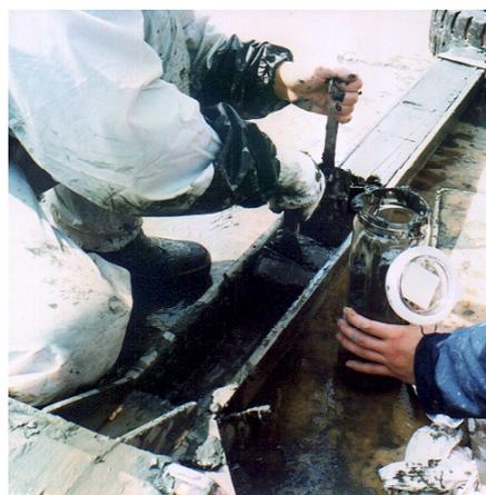
Figure 2. A core sample obtained from the sea bottom.
