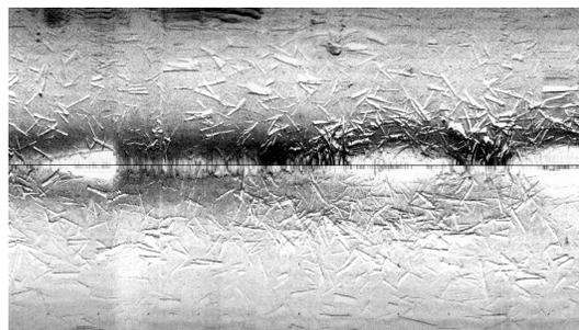
Fig. 2 Sidescan sonograph from Clio Bay showing dense concentrations of whole logs on the sea floor.
