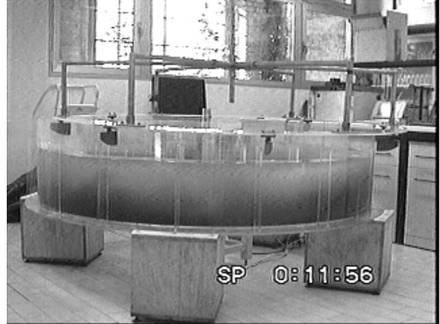
Figure 1. The Lab Carousel filled with seawater and sediments.
