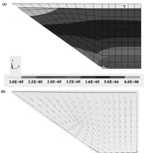
Figure 2 (A) Major principal effective stress distribution (in Pa) and (B) the deformation at the end of consolidation ( maximum principal stress :  $3.21 \cdot 10^5$  Pa at left bottom corner ; maximum displacement : 2.12 m at left top corner)
