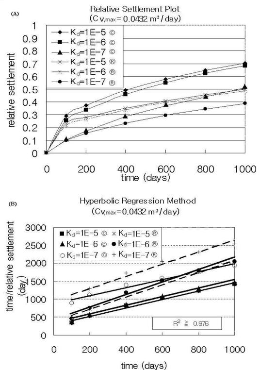
Figure 5 (A) Relative settlement in function of time and (B) its hyperbolic regression for the computation using “low value” range of the coefficient of consolidation (notations are the same to Figure 4)
