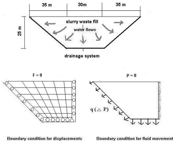
Figure 1. Model configuration and boundary conditions for the FE analysis (  $F$  : gravitational force ;  $P$  : excess pore pressure ;  $q(\Delta P)$  : flow rate at convective boundary)
