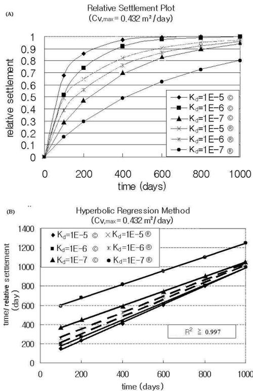
Figure 4 (A) Relative settlement in function of time and (B) hyperbolic regression, computed using “high value” range of the coefficient of consolidation;  $K_d$  : drainage hydraulic conductivity (m/sec);  $\odot$  indicates  $C_v$  constant ( $=C_{v,max}$ ) or decreasing with effective stress increased,  $\oplus$  indicates  $C_v$  increasing with effective stress increased
