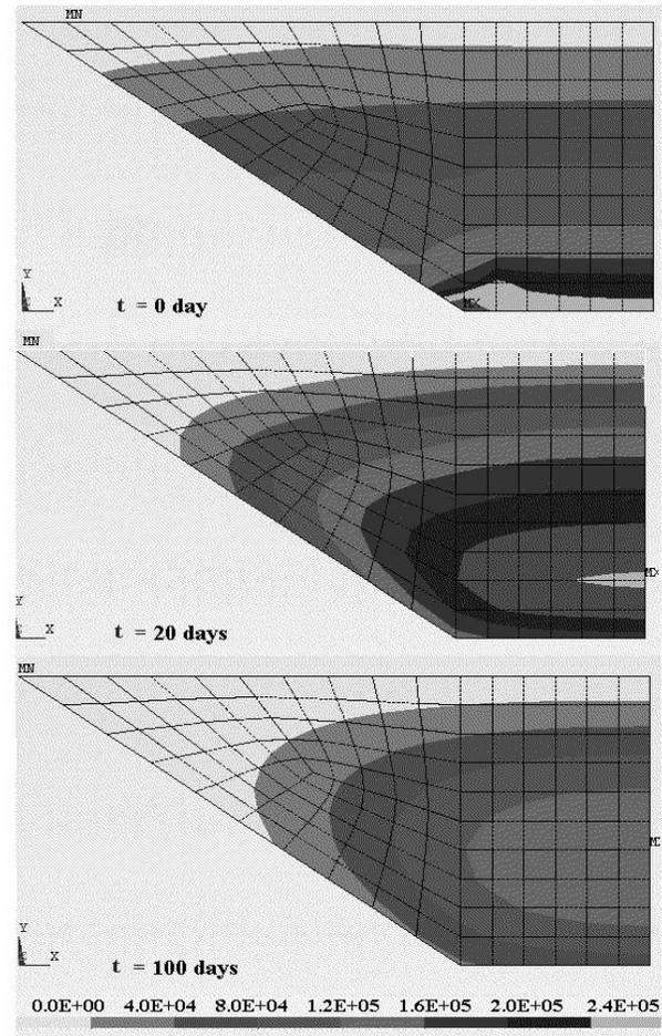
Figure 3 Excess pore pressure dissipation during consolidation (unit : Pa) ( $C_{v,max} = 0.432$  m<sup>2</sup>/day ;  $K_d = 10^{-6}$  m/sec) Top, middle and bottom figures show the distributions after 0 day, 20 days and 100 days, respectively.
