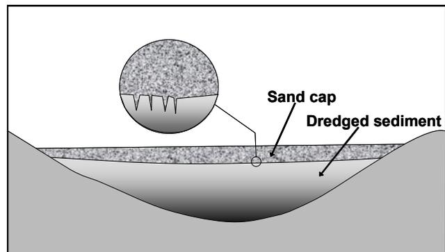
Figure 4. Final structure of the containment system after the cover layer has been placed (Oslo Harbour, 2001).
