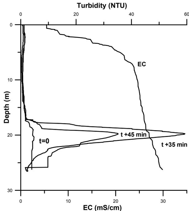
Figure 6. Change in turbidity profile after dumping of blast rock from a barge, the salinity profile shows the influence of the river water in the upper 5 m of the water column.
