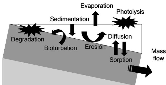
Figure 1. Main processes determining fate and transport of contaminants from sediments.
